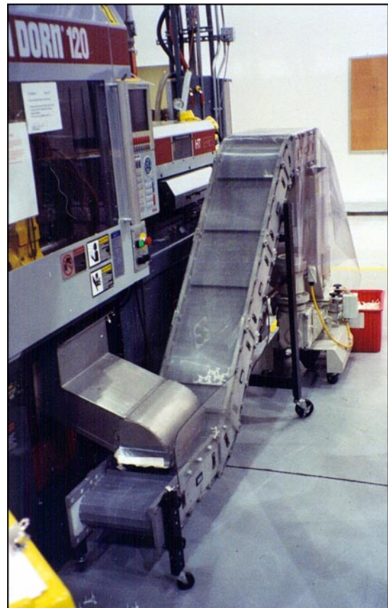
All four GW Plastics plants are standardizing utilizing DynaCon box filling and incline conveyor.
