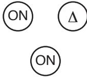
Press ON repeatedly until the display reads “end”, then press  $\Delta$ . See figure 5. The display will read “off”, then press ON and the display will go blank.
