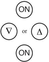
Enter Setup Mode (see page 2). Press ON repeatedly until the display shows “PIPE” (see Figure 10). Press  $\nabla$  or  $\Delta$  to change cooling line size. Available sizes are:
