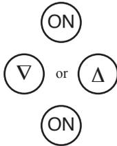
Enter Setup Mode (see page 2). Press ON repeatedly until the display shows “°F” or “°C” in the upper right corner and “unit” in the center. See Figure 6. Press  $\nabla$  or  $\Delta$  to change units. Press ON when desired unit is displayed.
