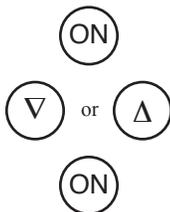
Enter Setup Mode (see page 2). Press ON repeatedly until the display reads “Auto” in the center. See Figure 8. Press  $\nabla$  or  $\Delta$  to change shut-off time (15 to 240 seconds). Press ON when desired shut-off time is displayed. Default value is 60 seconds.
