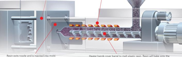
During a purge the nozzle is pulled back and resin is pushed out. Once the new resin comes out without any specks or streaking, the molding machine is put back into service. Heater bands cover barrel to melt plastic resin. Resin will bake onto the barrel and bits of old resin will flake off, which will impact quality. Over time resin "bakes on" barrel and screw.
