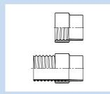
Soft sleeve to slide onto connectors or push into pipes, electrically conductive
