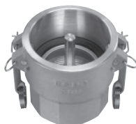
Aluminum Vapor Recovery Coupler with Probe; Female Coupler x Female NPT (with BUNA gasket & forged brass handles)
