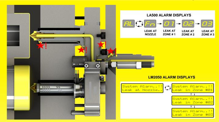
The AIRTECT Plastic Leak Alarm System is a unique device which gives protection against plastic leak damage caused by leaking plastic either within a Hot Runner Mold and/or at the IMM Injection Nozzle.
