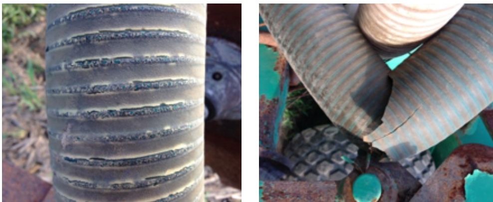
PVC Hose cracking due to UV exposure
