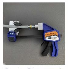
Slip the fitting onto the mandrel and begin moving the the movable section by squeezing the blue and black handles. Align the fitting into the end of the hose, continue slowly squeezing as the fitting is pressed into the hose up to the plastic washer.
