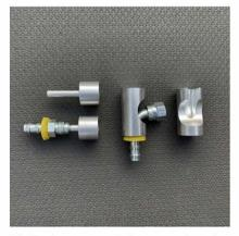
Select appropriate mandrel for your fitting installation and click it onto the stud on the movable section of the tool.
