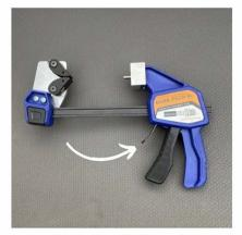
Open Barb-Tech IIc using the trigger release lever on the movable section of the tool.
