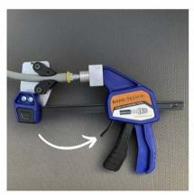
Release the pressure using the trigger release lever, slide mandrel out of the fitting, remove hose from the two spring loaded jaws by pulling out and forward toward the mandrel end.
