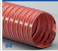
**Construction:** Double-ply silicone coated fiberglass fabric hose reinforced with a spring steel wire helix & external filament fiberglass cord.
