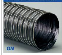
**Construction:** Double-ply neoprene coated fiberglass fabric hose reinforced with a spring steel wire helix & external filament fiberglass cord.
