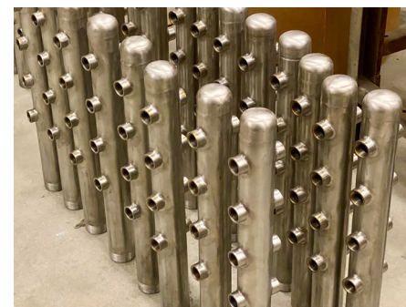
Tee Manifolds Awaiting Assembly for Brass Ball Valves. Application for Welding Gases for Car Manufacturer's Welding Robots (over 400 produced)
