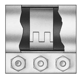
Gasket Protectors are for use with Morris Compression Couplings only and are not recommended for couplings less than 6" long.
