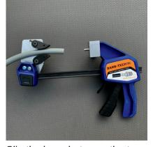
Slip the hose between the two spring loaded jaws with about 2 times the fitting barb length protruding beyond the jaws.
