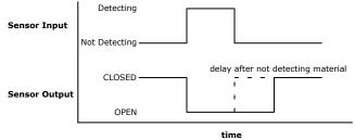
The sensors output is normally CLOSED.
