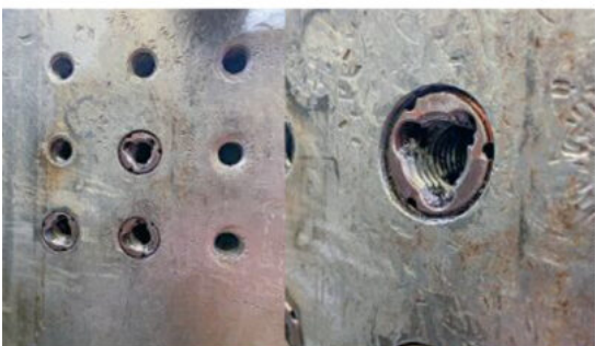
C-Sert threaded inserts help molders replace stripped bolt holes on platens with a new threaded hole that promises long service life.
