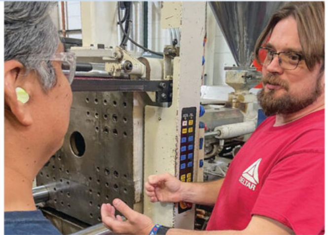
Kenny Dearing (right), ITW Deltar Fasteners process engineer, has utilized C-Serts to replace worn bolt holes on platens throughout the company's molding facility.
